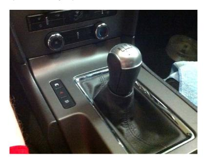
2. With the shifter in the neutral position, twist the shifter knob counter clockwise to remove. The knob may be really tight at first but will come loose without any added tools.
