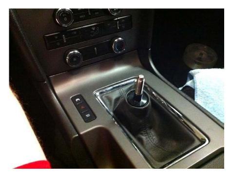
3. After the old shifter knob is fully removed, slide on the Shift Boot Retainer. There is an allen set screw installed in the groove that you will have to loosen. After you loosen the set screw, you can know slide the Shift Boot Retainer on.
