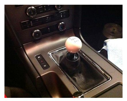
5. Now it's time to install the shifter knob. The knob should be screwed on clockwise. I used the supplied nut to get the shifter knob lined up properly.
