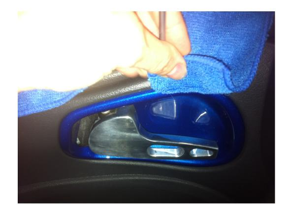
**3.** Detach the door speaker cover by pulling straight out. Now unscrew and remove the speaker assembly from the vehicle and unplug speaker electrical wiring clip.
