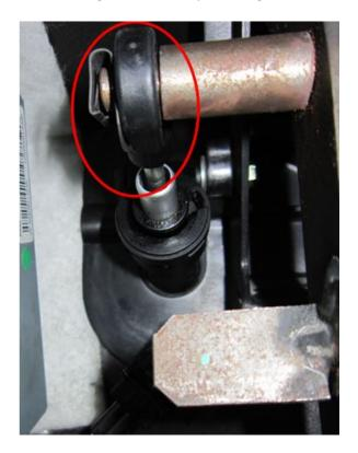
This will make your car immobile with no way to disengage the clutch. If yours is cracked, consider buying a new master cylinder to install along with the clutch line to avoid having to bleed the system multiple times.
