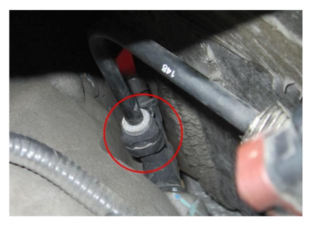
• Remove the clip here in the same fashion as you did at the top. A small pocketknife worked well to pry the clip loose in this limited space. Then pull the hose out of the fitting. The hose will now be free to remove from engine bay.
