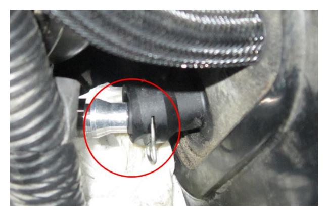
• Locate the transmission connection for the clutch line. This will be on the driver's side of the bellhousing, where the firewall slants back and narrows down to meet the transmission tunnel. You may be able to access this from below the vehicle, especially if you have removed the factory catalytic converters. I chose to access this from the top side, by reaching at an angle beginning at the driver's side cylinder head and down into the transmission tunnel.
