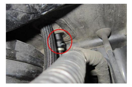
• Remove the metal clip securing the line to the firewall connection by prying the "looped" end out with a small flathead screwdriver. Be careful not to lose the clip, as it may pop out of the fitting.
