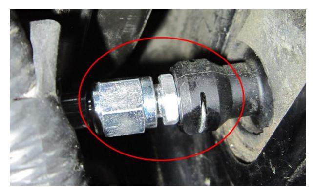
• Insert the other end of the hose into the transmission fitting. Secure it by fully re-inserting the metal clip. Long needle-nose pliers may be helpful for one or both of these steps.
