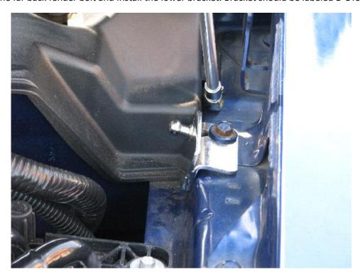
4. Remove the retaining pins from the strut and install on the upper bracket. Then remove the prop rod and lift the hood until you can install the bottom end of the strut on the lower bracket. Then reinstall the pins.
