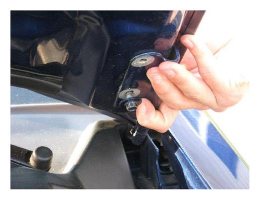
2. Slide the bracket labeled D-U (drivers upper) on the lower bolt and install the top bolt. There are probably dirt/paint lines where it used to be if the hood moved any when you removed the bolt. Try to line those up so you won't have to adjust the hood later. Tighten both the bolts down.
