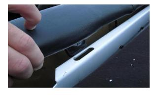
**Step 3:**Using a trim removal tool, remove the upper trim panel pin and the two rear trim panel pins that were hidden by the rear seat.
