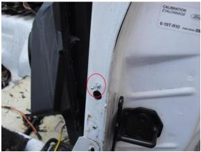
**Step 11:** Once the brackets are properly secured to the body of the vehicle, re-install the inner quarter panel trim and out trim panel by reversing Steps 3 & 4 above.
