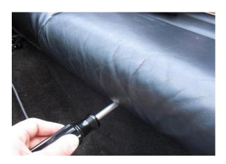
Step 2: Remove the two 10mm bolts holding the upper rear seat in place. Once removed, pull up on the seat to release the upper clips holding the seat to the vehicle.
