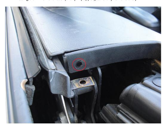
b. Remove the **two pins at the back/side** that were hidden by the seat back.
