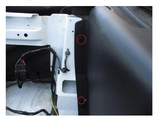
c. Very carefully remove the two small pins holding the rubber seal to the panel (at the top of the B-pillar)
