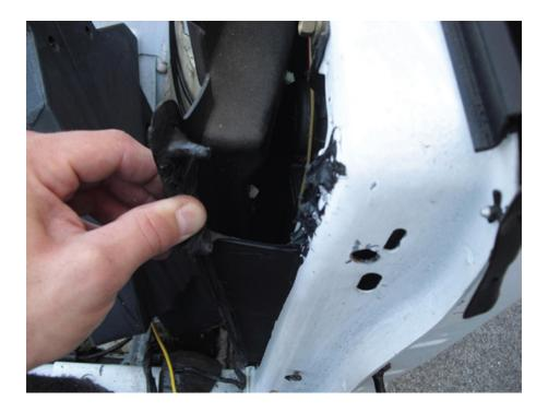
• Carefully pry the top of the cover out, and then pull the cover back – it does not need to be fully removed.
