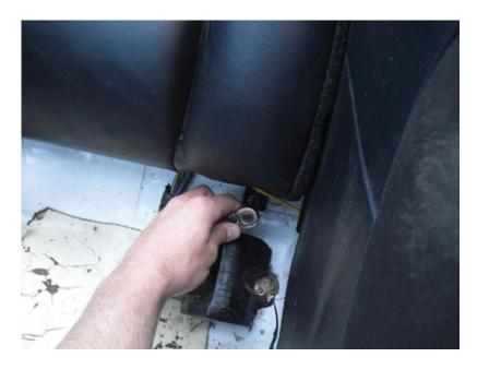
• Lift the seat back upwards until the two metal 'tabs' clear the vehicle body.
