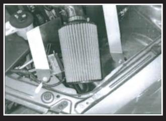
Install the air filter on to the end of the inlet tube. Push the filter over the inlet pipe until the stop in the filter is reached. Then install one hose clamp to secure the filter onto the inlet pipe.
