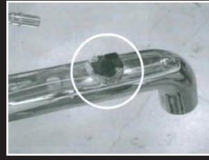
Check to be sure that the intake pipe is clear e. from debris. Install the MAF Sensor using the supplied mounting screws. Use Caution to avoid damaging the o-ring.
