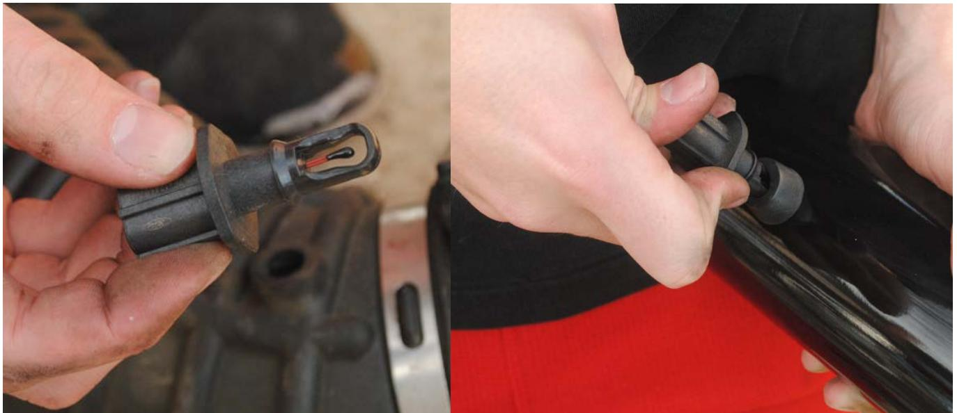
13. Take the upper 3" pipe and twist it into the coupler you installed on the throttle body. Twisting the pipe into place will insure a tighter fit.
