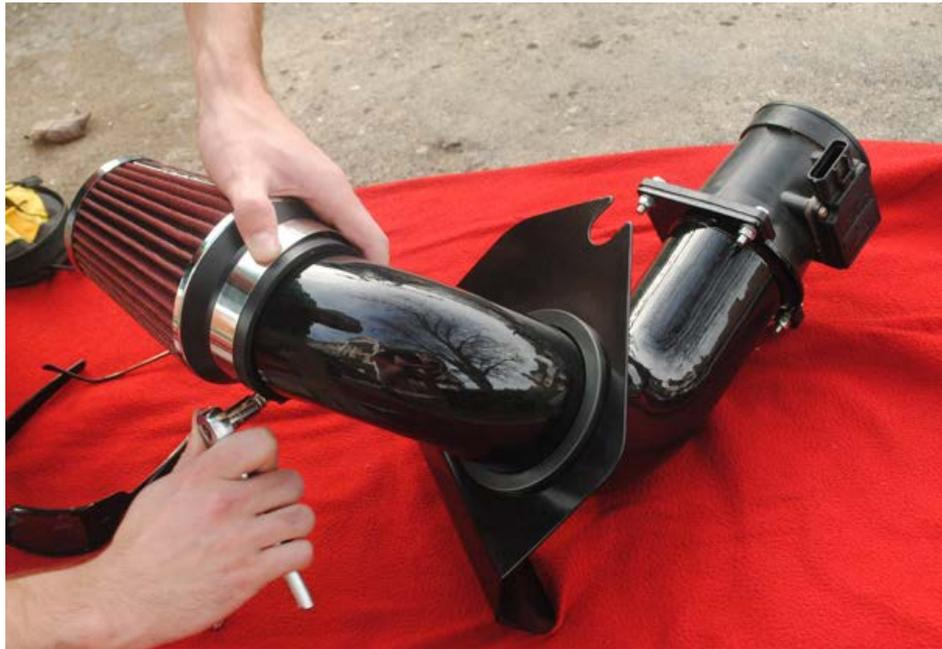
20. Slide the bottom half of the assembly into the fender, filter first.
