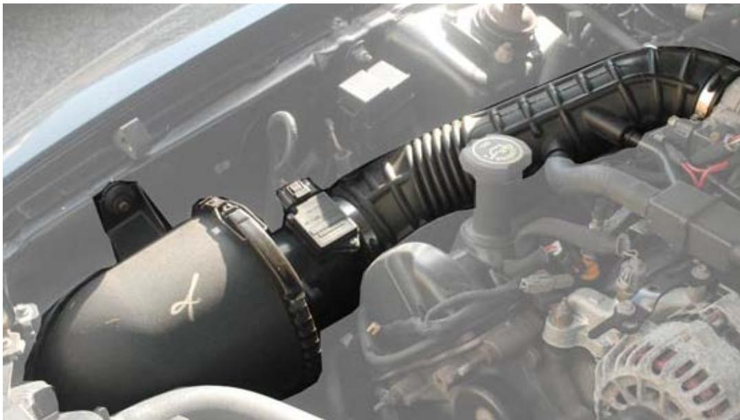
8. Remove the entire intake housing from the vehicle. This may require some wiggling and twisting, but it shouldn't be too hard to remove from the car.
