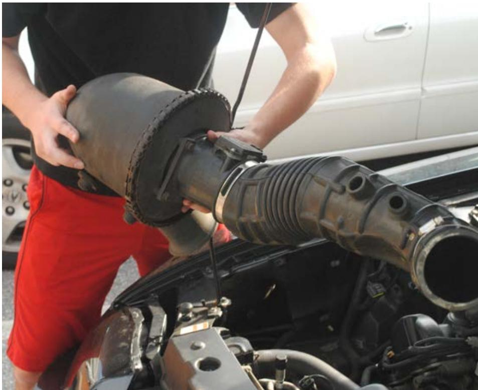
9. There should be (2) rubber grommets with the old intake housing that you removed. They may stay in place, but if they stay attached to the assembly, be sure to remove them and put them back onto the vehicle.
