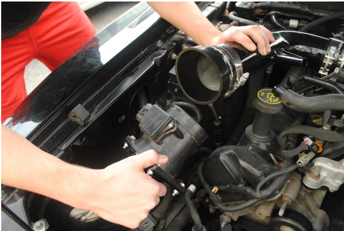
23. Make sure to do a double check on all bolts and clamps to make sure they are airtight.
