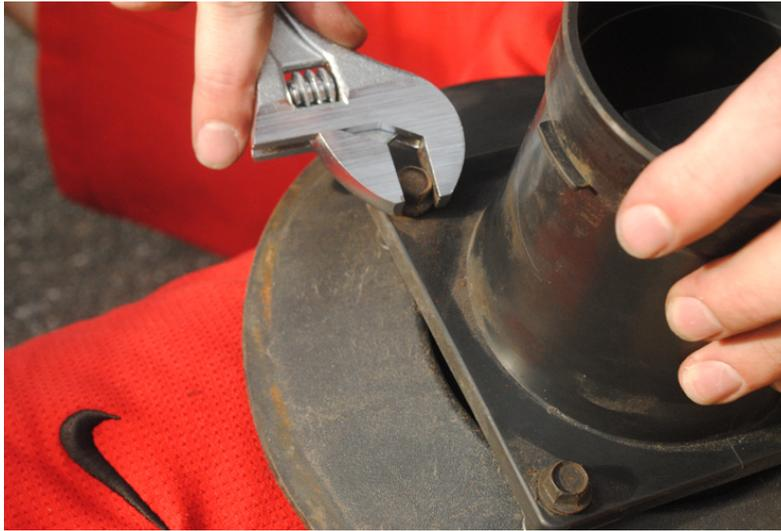
17. Using the parts provided in your kit, use an 11mm socket or an adjustable wrench to assemble the Mass Air Flow sensor to the kit's 3.5" pipe. Be careful not to tighten the bolts too much or you will crack the MAF's housing. You will need the gasket, (4) 1" bolts, (4) Nylon Lock Nuts and \*4) Small washers for assembly.
