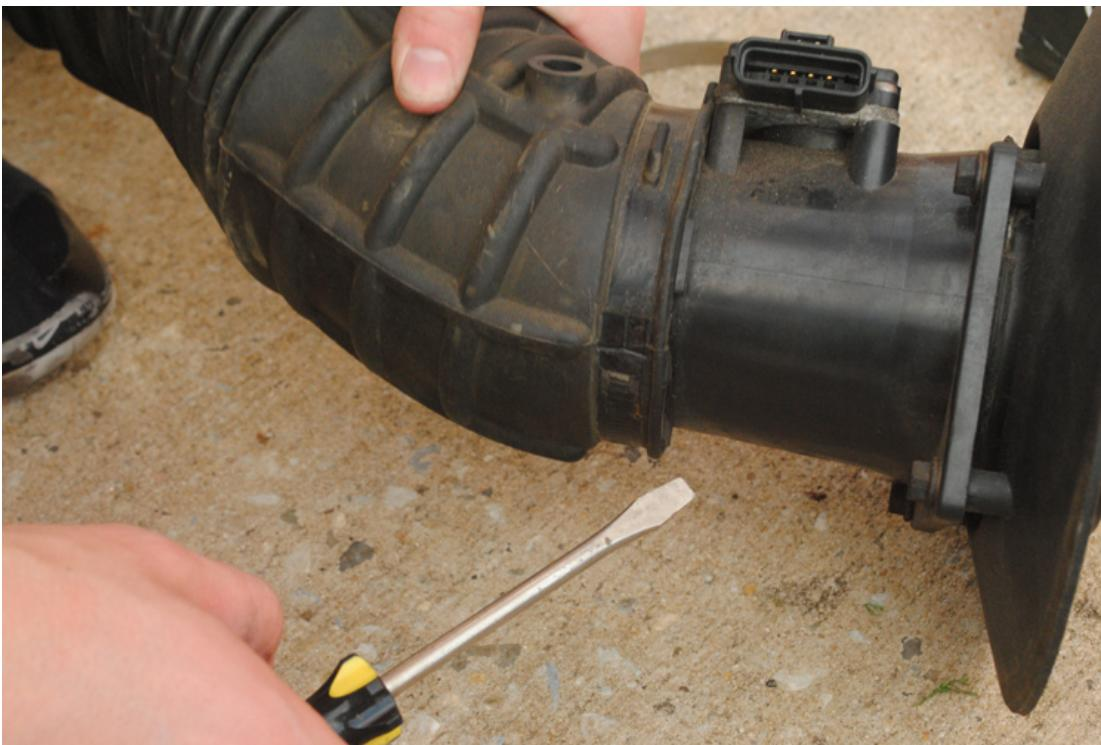
16. Remove the (4) bolts around the base of the sensor and you will have the part you need.
