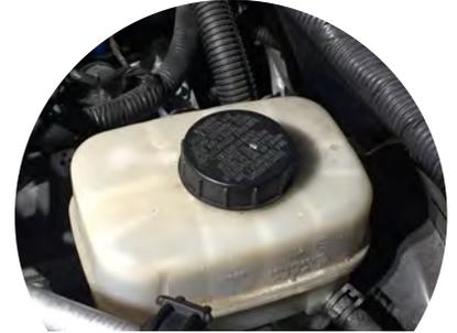
**Brake Fluid Reservoir Cap:** Using the supplied alcohol wipe, clean the reservoir cap. Ensure the cap is tight. Test Fit the Modern Billet cap. Loosen the set Allen screw(s). Remove the double sided tape backing, place the cap over the reservoir and tighten the set screw(s).
