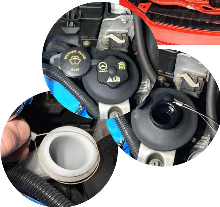
**Windshield Reservoir / Power Steering Cap:** Remove the factory reservoir cap. Wrap the cable tether around the reservoir opening then press the cap onto the reservoir.
