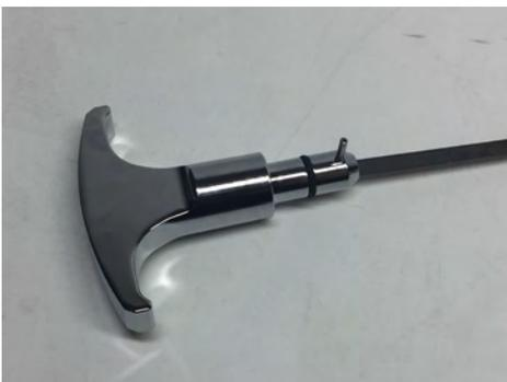
Re-install the factory roll pin in the Modern Billet handle.
