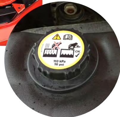
**Radiator Cap Cover:** Using the supplied alcohol wipe, clean the reservoir cap. Ensure the cap is tight. Test Fit the Modern Billet cap. Loosen the set Allen screw(s). Remove the double sided tape backing, place the cap over the reservoir and tighten the set screw(s).
