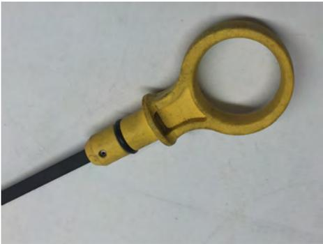
Remove the dipstick from the vehicle. Using an appropriate sized punch or drill bit, tap out the factory roll pin.
