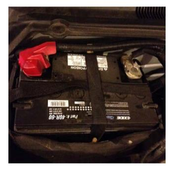
5. After locating the battery connect the black lead first than connect the red lead. If electric makes your nervous don't be, this battery butler is very safe the leads don't spark if they accidently touch. Also the leads have a rubber hose on them for your protection.
