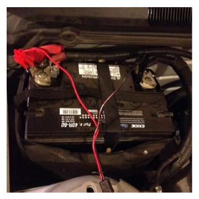
6. Now that the leads are connected & the battery butler is already connected to a power source! The green charging light will turn on. At this point all your worries about having a dead battery are over! The battery butler is already doing its job of keeping the battery charge at what it should be & not over charging it.
