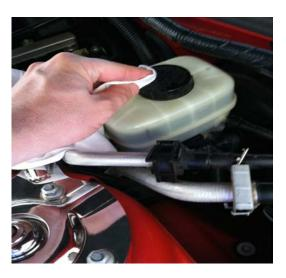
(2) Remove 3M Tape and press Cap Cover onto Plastic Brake Fluid Cap
