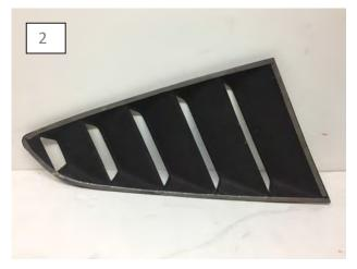
Apply the supplier double sided tape to the back of the window louver as shown.
