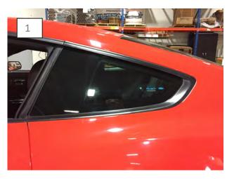
Thoroughly clean the quarter window to ensure the cleanest possible surface. \*\*Note: Isopropyl alcohol will help remove any paint contaminates. Allow the window plenty of time to dry.
