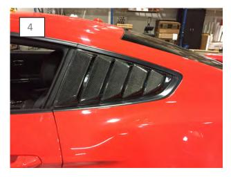
Apply firm pressure to tape locations to ensure proper adhesion.
