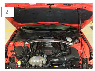
Place the Carbon Fiber Engine Cover onto the motor. Apply pressure to ball mount location to clip the cover into the rubber mounts. Reinstall strut tower brace in reverse order.
