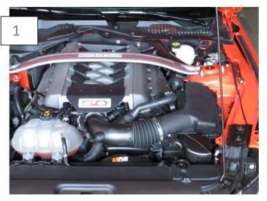
Begin by removing the engine cover. Firmly pull on the corners to dislodge the cover from its rubber mount. \*\*Note: If equipped with factory strut tower brace remove the (4) 15mm bolts securing the brace to the vehicle.
