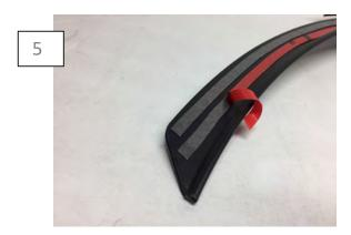
Peel off the tape backing prior to installing the winglet.
