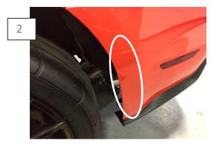
Thoroughly clean the back side of the bumper cover to remove any and all wax/grease. \*\*Note: Use isopropyl alcohol to ensure the cleanest possible tape surface.
