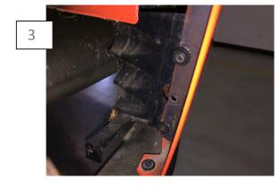
Using a 7mm socket, remove the (2) bolts securing the bumper cover to the bumper bracket. \*\*Note: This hardware will be used when installing the winglet.
