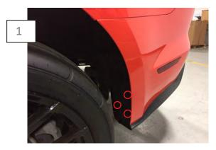
Remove the (3) fender liner clips and fold the fender liner out of the way.
