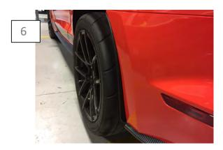
Using the factory hardware, bolt the winglet to the vehicle. Apply firm even pressure to the taped surface to ensure proper adhesion.
