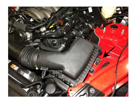
Step 4: Slide back the red locking clip on the MAF sensor plug. Then depress the locking tab to remove the plug from the sensor. Use a pry tool to remove the wiring harness retaining pin from the air box.
