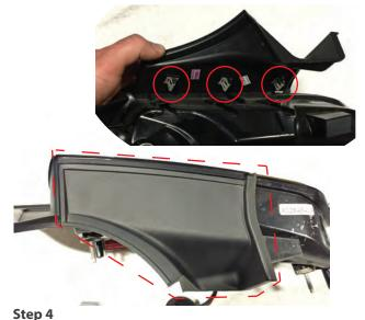
Remove the upper plastic trim panel from the factory tail light. Use a plastic trim removal tool and gently pry upward.
