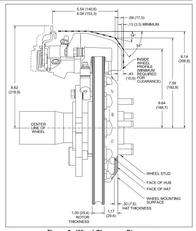
Figure 2. Wheel Clearance Diagram
