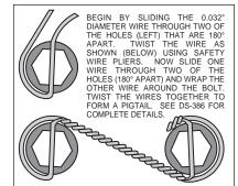
Figure 3. Safety Wire Diagram
