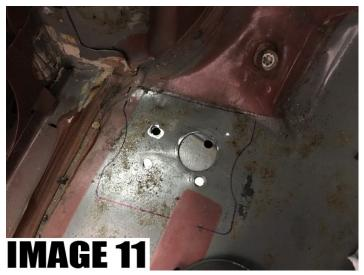
If welding, continue to steps 10 - 12. NOTE: If welding plates, use caution not to melt wiring harness or grommet.
