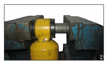
20. Place one of the coil springs onto the lower spring perch. Position the lower spring perch so that the top of the spring is well below the welded isolator bung on the shock piston rod, as this will make the installation of the remainder of the parts much easier.
