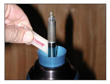
25. Place one of the Delrin pivot balls on the shock piston rod with the curved side facing down toward the aluminum pivot socket.
