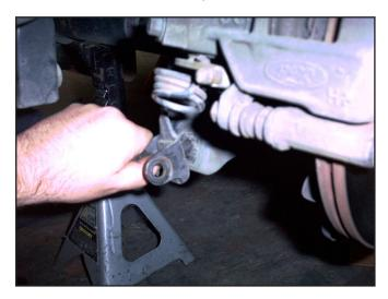
15. Install the MM lower shock mount onto the passenger side of the axle. Insert the 1/2" bolt (no washer) through the lower hole, with the bolt head facing the rear of the car. Next, place the
