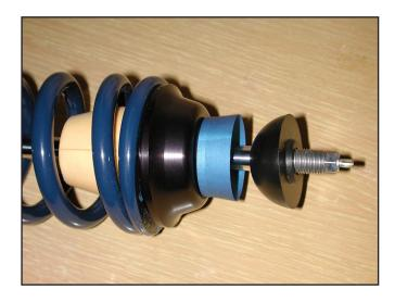
You have now completed one coil-over assembly. Repeat Steps 16 - 25 for the second shock absorber.
