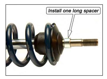
36. Place the strut shaft top into the spherical bearing of the C/C plate. Tighten the strut top retaining nut with enough spacers on top of the spherical bearing to prevent the nut from running out of threads on the strut shaft.
