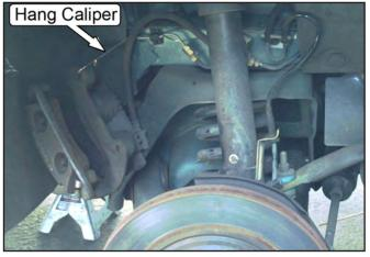
5. While it is not necessary, you may find it helpful to remove the brake rotor. Disconnect the outer tie-rod end from the spindle.
