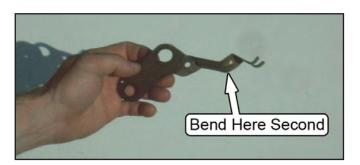
49. Reattach the mounting bracket to the spindle and adjust the bends if necessary to keep the mounting bracket close to the strut. Install and tighten the retaining nut for the mounting bracket.
