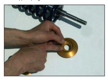
32. Place one Needle Bearing Race into the recess on the top side of the Upper Spring Perch. Completely pack the Thrust Needle Bearing with a high quality Moly wheel bearing grease. Place the Thrust Needle Bearing on top of the installed Needle Bearing Race. Place the second Needle Bearing Race on top of the Thrust Needle Bearing.
