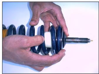
NOTE: Some companies C/C plates have a fixed-type spacer bushing pressed into the spherical bearing. With these types of C/C plates, skip Step 35, and you may not be able to maximize bump travel in Step 40.
