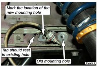
Move the brake line bracket out of the way and drill a 1/8" diameter hole on the mark made in Step 4. (Figure 3)
