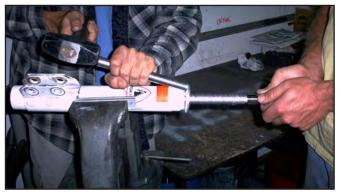
19. The collar will stretch around each spot-weld before breaking. Rotate the strut in the vise, hitting each spot weld evenly to avoid excessively tipping the collar and gouging the strut shaft.
