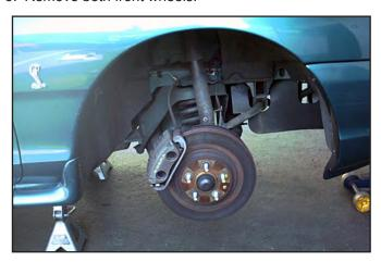
4. Unbolt the brake caliper and hang it securely. Do not let the caliper hang from the brake hose, as this can cause unseen damage to the hose. Steel braided hoses are especially susceptible to damage if the caliper is dropped or allowed to hang unsupported.
