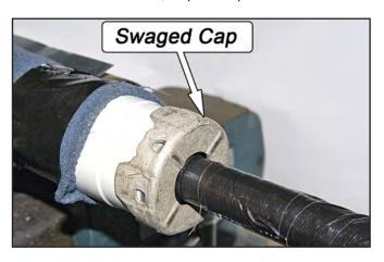
18. If you are using Tokico struts, you must remove the upper flange from the strut. To do so, place the strut in a vise with soft aluminum jaws. Clamp the strut firmly but not so tight as to distort the housing. Generously duct tape the strut shaft to prevent damage. Have a friend support the end of the strut to keep it from dropping under impact. Use a hammer and a large drift to break the spot welds on the flange.
