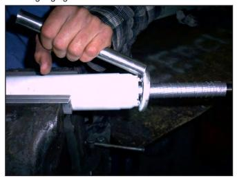
20. Once you have broken all three spot welds, remove and discard the Tokico upper flange.
