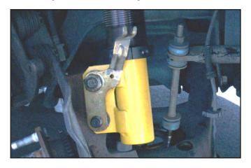
50. Clean any dirt from the tip of the ABS sensor and reattach the ABS sensor to the spindle. Reattach the sensor's wire to the mounting bracket.
