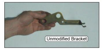
47. Use two sets of pliers to hold and bend the bracket forward near the base.
