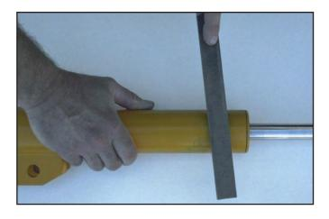
26. Slide the threaded sleeve down over the strut housing, unthreaded end first, until the notch in the bottom of the sleeve straddles the ears of the strut.
