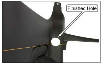
46. Cut the plastic quarter panel into two pieces, along the line that was drawn, using a wood saw or other cutting device.
