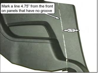
44. At the bottom of the quarter panel, extend the line across the horizontal flat. Add a mark about 3/8" forward of the line, centered side-to-side on the flat section.
