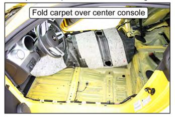
**NOTE:** If present, disconnect the wiring harness connected to the seat belt so that the carpet can be folded over the center console.
