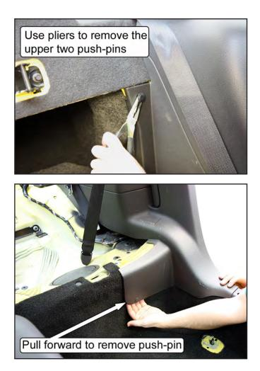
12. Remove both front plastic kick panels. Pull the portion closest to the firewall inboard to disengage the push-pin retainer, and then pull the panels rearward.
