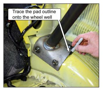
Remove the sound-deadening material within the outline using a chisel or other scraping device.
