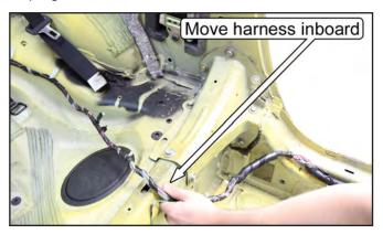
**NOTE:** There is a release clip that must be disengaged on the inboard face of the seatbelt retractor electrical connector on some vehicles. Use a small screwdriver to pop the release clip up, away from the connector.
