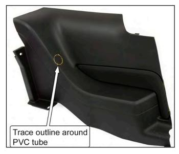
53. Remove the rear half of the plastic panel from the vehicle and hole saw through the location marked for the rear support. Use a 2" hole saw if available, or you can use a 1-3/4" hole saw to file the opening out larger.
