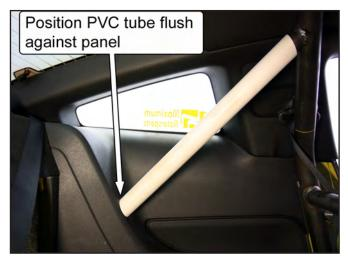
52. Use a marker to trace around the PVC tube, the location where the rear support will pass through the plastic panel.
