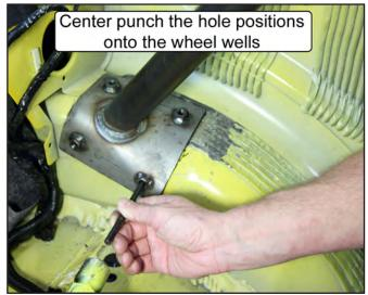
35. Mark the position of the four mounting holes in each door bar mounting pad onto the floor pan using a center punch.
