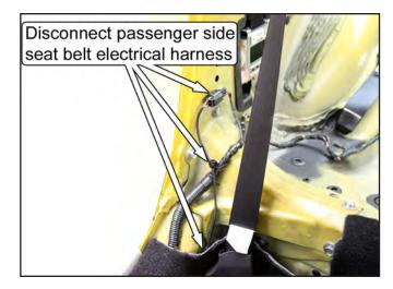
15. Relocate the wiring harness in the area adjacent to each B-pillar. Unfasten the harness retaining clips and pull the harness inboard to clear the factory support brackets. If necessary, get more slack by disconnecting the harness where it plugs into each of the seat belt retractors.
