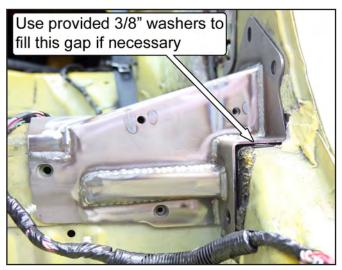
20. Check the gap between the bracket and the vehicle at H8. Use the provided 3/8" G8 washers to close the gap to 1/8" or less. When satisfied, insert one of the factory mounting bolts into the hole to prevent the washers from dislodging.
