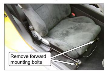
Tip the seat back to disconnect the wiring harness connectors for the air bag module and seat. Carefully pull the seats out of the car and place aside.
