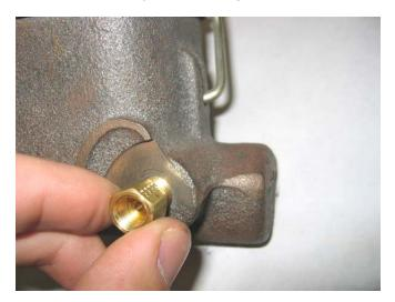
2. Place the larger, 9/16" adapter into the rear port of the master cylinder and tighten to 12-16 ft-lbs.
