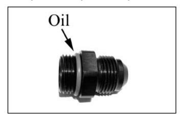
10. Place the Remote Filter Mount into a vise with "soft jaws" and install each of the two Straight Thread O-ring to -10AN fittings into the two ports of the filter adapter. Tighten the adapter nipples to 35 ft-lbs.
