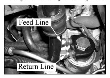
40. Use the supplied zip ties to secure the oil lines as needed.
