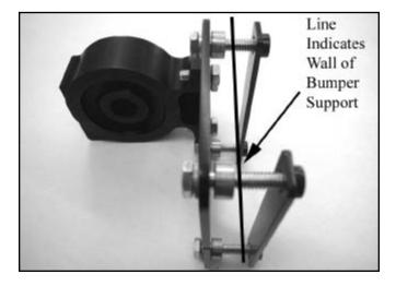
15. Tighten all four adapter plate bolts to 10 ft-lb. Note: While the photo below shows the oil lines already installed, they should not be installed until Step 22. (Braided steel lines shown)
