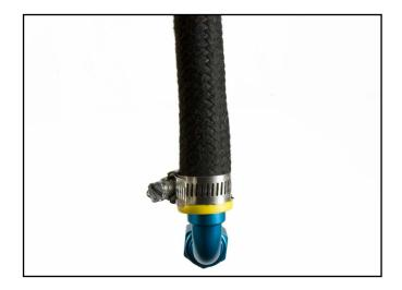
22. Hand tighten the attached 90-Degree fitting onto the adapter nipple of inboard port of the Remote Filter Mount (the adapter nipple closest to the radiator support).
