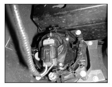
5. Position the Adapter Plate on the bumper support, and use it as a template to locate the position of the required four new mounting holes on the bumper support. Make sure that the top of the plate is lower than any protrusions from the overhead plastic panel, and that each new hole location has at least 1/8" of metal between it and any OEM holes in the bumper support.
