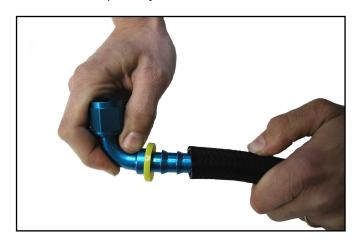
21. Slide a hose clamp over the end of the hose that does not have a fitting. Position the hose clamp next to the yellow hose end cover and then use a slotted screwdriver to tighten the clamp until snug. The hose clamp provides extra security in high heat and pressure applications.
