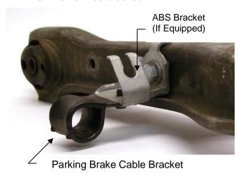
6. Loosen the lower control arm pivot bolts, 2 bolts per control arm.
