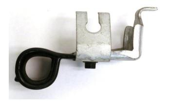
13. Flip the Parking Brake Bracket 180 degrees and place the ABS bracket on top of the Parking Brake Bracket.
