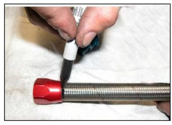
22. Use motor oil to lubricate the threads and the tip of the blue nipple that will be inserted into the hose. Use motor oil to lubricate the inside and cut end of the hose. Place the blue nipple in a vise. Hold the HOSE (not the red socket), and push the hose onto the blue nipple far enough to engage the threads of the red socket. Turn the HOSE to thread the red socket onto the blue nipple. Tighten as far as possible by hand.
