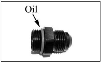
10. Place the Remote Filter Mount into a vise with "soft jaws" and install each of the two Straight Thread O-ring to -10AN fittings into the two ports of the filter adapter. Tighten the adapter nipples to 35 ft-lbs.
