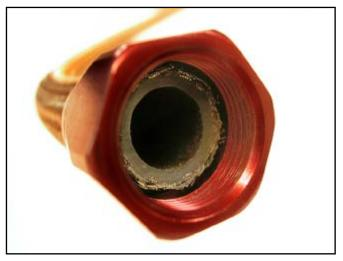
21. Use a felt-tip pen to mark the hose at the base of the socket, so that you can tell if the hose is getting pushed out during the remaining steps of the fitting installation.
