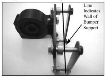
15. Tighten all four adapter plate bolts to 10 ft-lb. Note: While the photo below shows the oil lines already installed, they should not be installed until Step 22.
