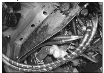
41. Use the supplied zip ties to secure the oil lines as needed.
