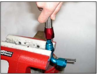
23. When you can no longer tighten the fitting by hand, use appropriate size wrenches to tighten the fitting. Tighten the fitting until the red socket is within 1/16" from bottoming on the blue nipple. Do NOT use adjustable or oversize wrenches, or you will damage the fitting.
