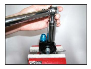
11. Attach the Adapter Plate to the Remote Filter Mount using the three supplied 5/16" bolts. Orient the plate so that the Remote Filter Mount will be biased toward the fender when installed on the car. Tighten the three bolts to 19 ft-lb.
