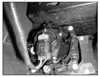
Position the Adapter Plate on the bumper support, and use it as a template to locate the position of the required four new mounting holes on the bumper support. Make sure that the top of the plate is lower than any protrusions from the overhead plastic panel, and that each new hole location has at least 1/8" of metal between it and any OEM holes in the bumper support.
