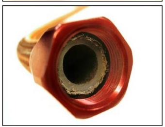
20. Use a felt-tip pen to mark the hose at the base of the socket, so that you can tell if the hose is getting pushed out during the remaining steps of the fitting installation.
