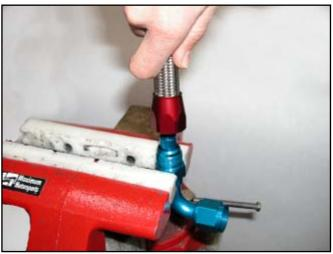
22. When you can no longer tighten the fitting by hand, use appropriate size wrenches to tighten the fitting. Tighten the fitting until the red socket is within 1/16" from bottoming on the blue nipple. DO NOT use adjustable or oversize wrenches, or you will damage the fitting.
