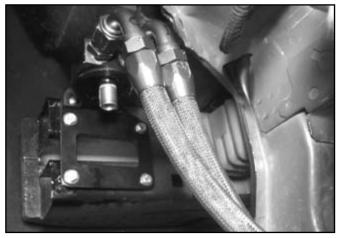
37. Fine tune the orientation of the Engine Block Adapter in order to give the best oil line routing. The block should be oriented such that the oil lines are positioned as far away from the swaybar as possible without interfering with the steering rack boot, similar to the OEM power steering line routing. Tighten the Engine Block Adapter to the engine.
