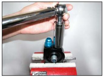
11. Attach the Adapter Plate to the Remote Filter Mount using the three supplied 5/16" bolts. Tighten the three bolts to 19 ft-lb.
