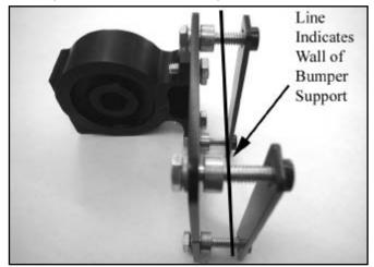
15. Tighten all four adapter plate bolts to 10 ft-lb. Note: While the photo below shows the oil lines already installed, they should not be installed until Step 35.
