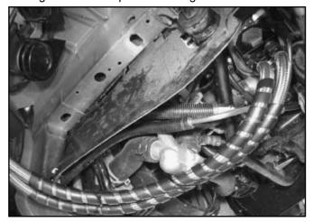
WARNING: Braided steel line is very abrasive. Normal engine and driving vibrations will cause it to wear through other items near it if it is not properly insulated.
