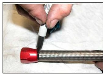
21. Use motor oil to lubricate the threads and the tip of the blue nipple that will be inserted into the hose. Use motor oil to lubricate the inside and cut end of the hose. Place the blue nipple in a vise. Hold the HOSE (not the red socket), and push the hose onto the blue nipple far enough to engage the threads of the red socket. Turn the HOSE to thread the red socket onto the blue nipple. Tighten as far as possible by hand.
