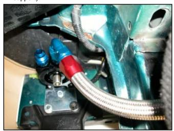
25. Route the hose under the frame rail, under the antisway bar, and up to the Engine Block Adapter. The specific routing should be based on your personal preference and vehicle configuration.
