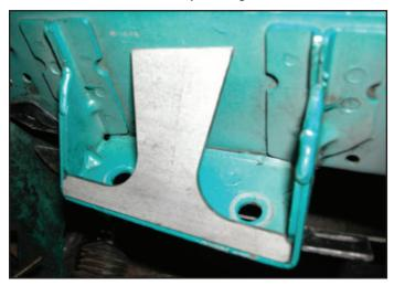
8. Mark with a Sharpie pen or grease pencil all areas where the MM Reinforcement contacts the frame rail.
