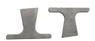
The 1979-93 Mustang front swaybar mount is spot welded into place. Because it hangs off the frame rails, it is prone to flexing and commonly develops cracks. The MM Front Swaybar Bracket Reinforcement braces the factory swaybar mount to prevent flexing and stop cracks from developing.
