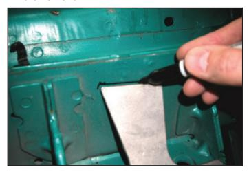
9. Remove the MM Reinforcement. Wire wheel or sand, to bare metal, all areas to be welded.
