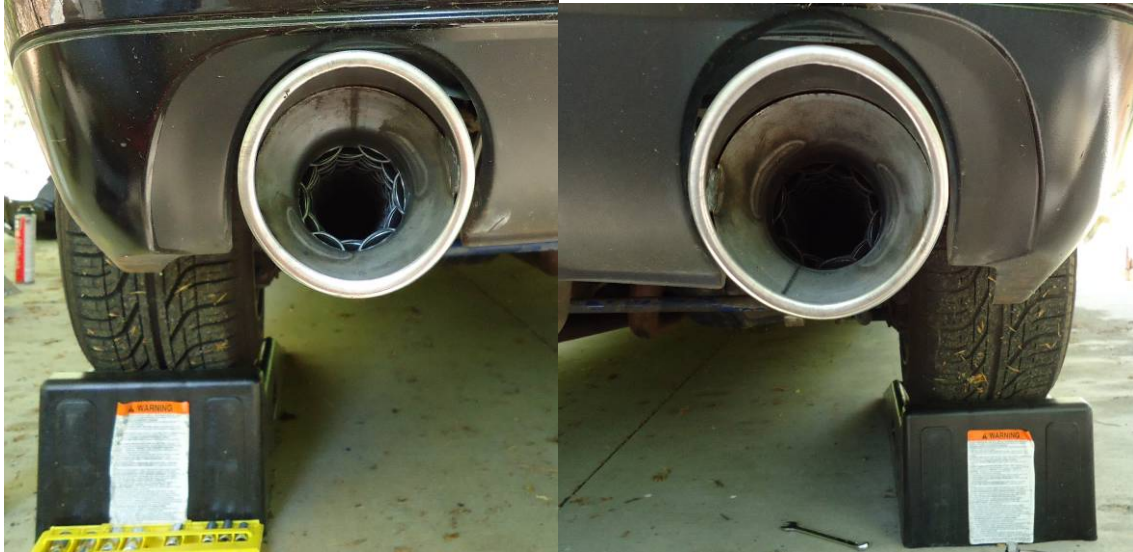
The Passenger Side Exhaust Tip is Too Low
