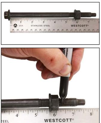
88. Use a hack saw or grinder to cut each bolt at the mark placed in Step 87.
