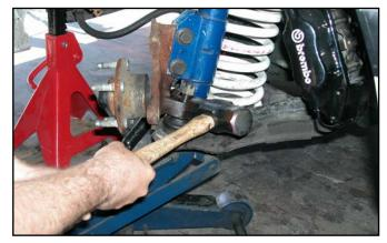
23. For cars equipped with conventional front coil springs, use an internally mounted coil spring compressor and compress the front coil spring. Most auto part and equipment rental stores rent this type of spring compressor.
