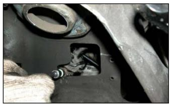
32. Remove the two bolts that hold the steering rack to the K-member. Pull the steering rack forward until it is just below the swaybar. To keep the steering rack out of the way, zip tie or wire it underneath the swaybar. It is not necessary to disconnect any hoses from the steering rack.
