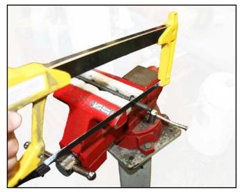
89. You will need to chamfer the edges of the cut bolts and clean the threads with a file so the OEM Ford nuts will easily start to thread onto the bolts. The bolt thread is M12 x 1.75. If you have a thread file or a die set, this can be used to clean up the threads after a chamfer has been put on the end with a file. After the bolt tips are dressed, remove the nuts as the final Step to ensure the threads are properly formed.
