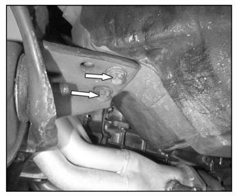
38. Remove the four bolts near the spring pockets completely. Have a second person stabilize the K-member while doing this. Slowly lower the floor jack and K-member while also checking for any objects that may hang up on the K-member. Lower the K-member to the floor and remove it from underneath the car.
