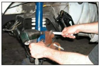
14. Loosen the tie-rod end nut but do not remove it.
