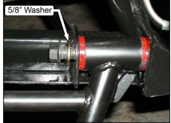
81. Thread a factory nut onto each pivot bolt.
