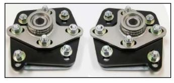
101.Install a front coil-over conversion kit now if the car is not yet so equipped.
