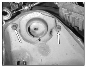
37. Remove the four bolts at the rear of the K-member.
