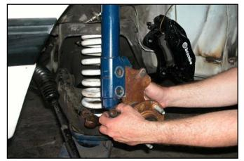
27. For easier access, remove the strut from the car.
