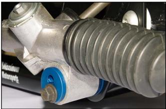
93. Check the orientation of the clamps which secure the rubber rack bellows boots to the rack housing. If the clamp bolt is installed towards the K-member as shown below, the clamp bolt may prevent the steering rack from being fully seated against the K-member. If necessary, rotate the position of the boot clamps.
