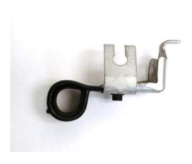
13. Flip the Parking Brake Cable Bracket 180 degrees and place the ABS Bracket on top of the Parking Brake Cable Bracket.
