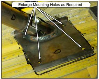
NOTE: There ARE fuel and brake lines directly beneath the driver side Door Bar Mounting Pad. Take care when enlarging the holes that the lines do not get damaged.
