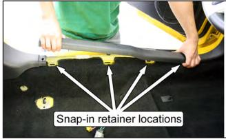
4. Remove both front plastic kick panels. Pull the portion closest to the firewall inboard to disengage the push-pin retainer, and then pull the panels rearward.
