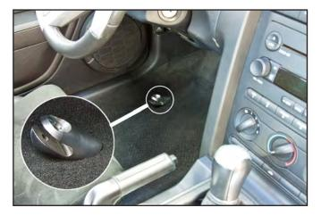
14. Install the plastic kick panels and secure each one with a plastic push-pin.
