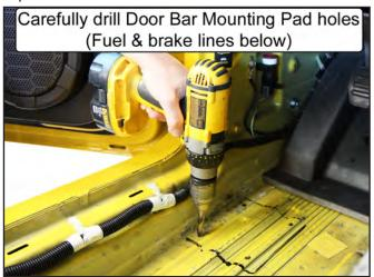
**NOTE:** There ARE fuel and brake lines directly beneath the driver-side door bar mounting pad. Place the door bar doubler plate between the underside of the floor pan and the lines (as a shield) when drilling to prevent puncturing the lines.
