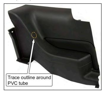
53. Remove the rear half of the plastic panel from the vehicle and hole saw through the location marked for the rear support. Use a 2" hole saw if available. If not, you can use a 1-3/4" hole saw and file the opening out larger.
