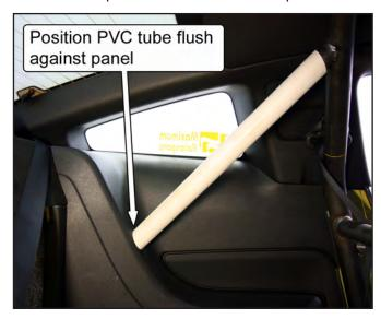
52. Use a marker to trace around the PVC tube, the location where the rear support will pass through the plastic panel.
