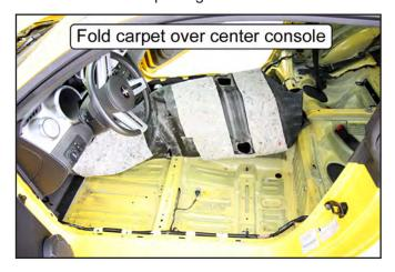
**NOTE:** If present, disconnect the wiring harness connected to the seat belt so the carpet can be folded over the center console.
