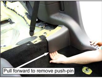
12. (DB ONLY) Remove both front plastic kick panels. Pull the portion closest to the firewall inboard to disengage the push-pin retainer, and then pull the panels rearward.
