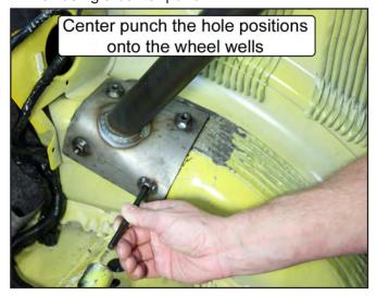
35. (DB ONLY) Mark the position of the four mounting holes in each door bar mounting pad onto the floor pan using a center punch.
