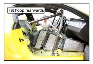
27. Trace an outline of the rear support mounting pads onto the driver- and passenger-side wheel well, and then remove the roll bar from the vehicle.
