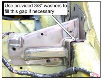
20. Check the gap between the bracket and the vehicle at H8. Use the provided 3/8" G8 washers to close the gap to 1/8" or less. Then insert one of the factory mounting bolts into the hole to prevent the washers from being dislodged.
