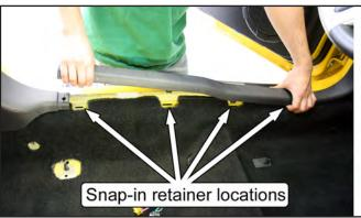
11. Remove the rear quarter panels. There are three push-pin retainers on each panel; one is located at the front of the seat bulkhead and two are at the rear seat backrest. Carefully pull the rear half of the panels inward to disengage the snap-in retainers located below the quarter window, and then pull the panels forward.
