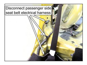
15. Relocate the wiring harness in the area adjacent to each B-pillar. Unfasten the harness retaining clips from the vehicle and pull the harness inboard to clear the factory support brackets. If necessary, you can get more slack by disconnecting the harness where it plugs into each of the seatbelt retractors.
