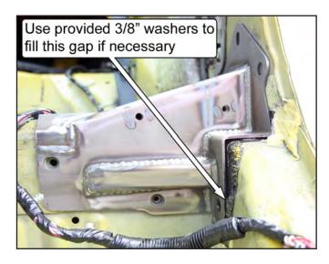
21. Install the remaining mounting bolts into the support bracket and tighten them by hand. Take note that H6 and H7 use the larger, 15mm hex head bolts.
