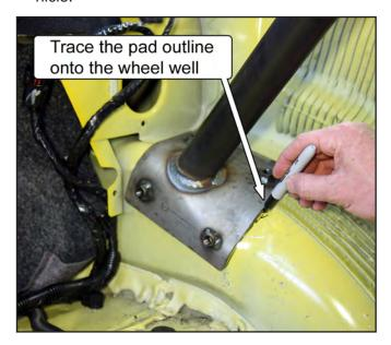
28. Remove the sound-deadening material within the outline using a chisel or other scraping device.
