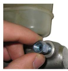
2. Place the remaining two smaller, 10mm adapters into the two rear ports of the master cylinder and tighten to 12-16 ft-lbs. One port is located on the inner side of the master cylinder, and the other port is located on the underside of the master cylinder.
