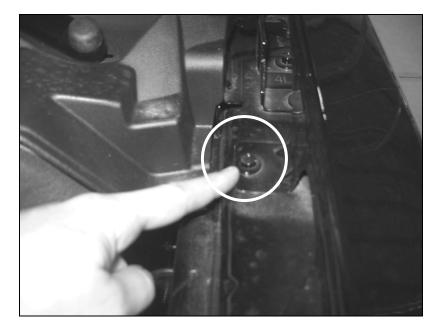
5. Install the left hand fender bracket (1312-LHFNDR), re-install the factory bolt and torque to 20 Nm.
