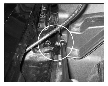
13. Raise the hood upward (to increase travel) and insert the opposite end of the strut onto the hood mounting brackets on either side.
