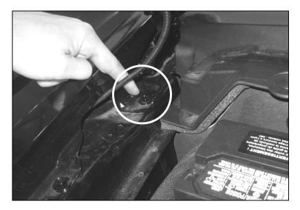
3. Install the right hand fender bracket (1312-RHFNDR) as shown, re-install the factory bolt and torque to 20 Nm.
