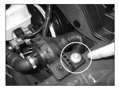
2. Remove the steel reinforcement insert from the rubber grommet. Note - Tube was removed from vehicle for clarity. This modification can be completed with the tube in vehicle position.
