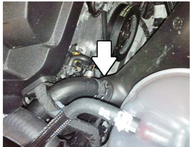
11. Remove the PCV quick connect fitting from the stock clean air tube.
