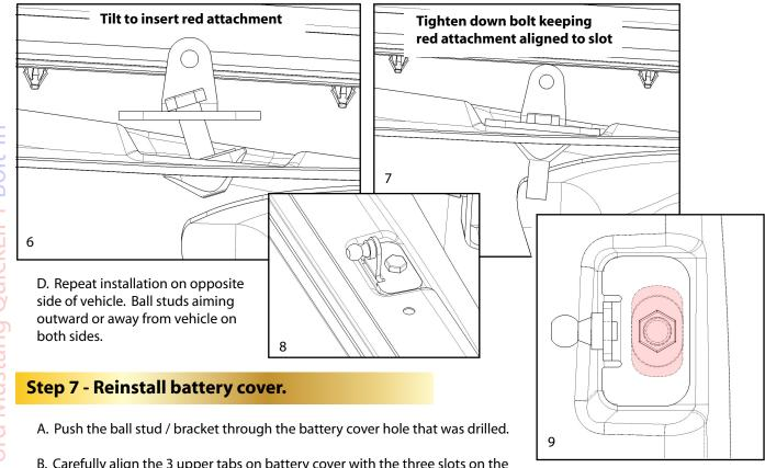
B. Carefully align the 3 upper tabs on battery cover with the three slots on the cowl. Slide cover into slots and then reinstall the push pins into the front of the battery cover. *Be sure that the cover gets tucked back around the battery cables and is fully seated.*
