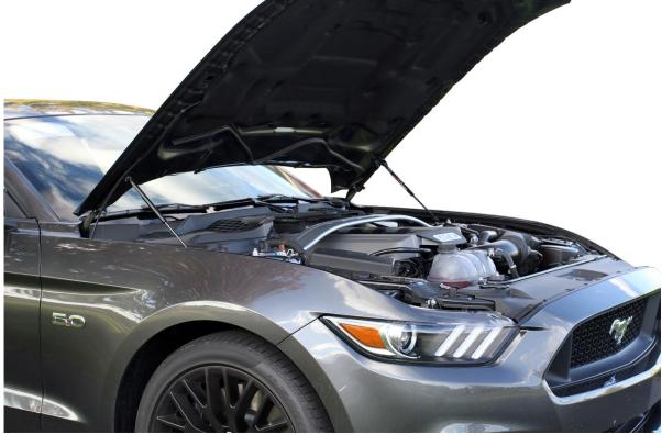
How To Remove Struts: Slide a small flat blade screw driver under the metal c-clip. Lift and rotate c-clip (DO NOT REMOVE C-CLIP). Gas spring will pop off of ball-stud.
