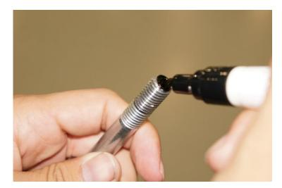
20. To Transfer the Hole to the inside of the Channel on the back of the Bumper Beam, apply some paint to the end of the Bolt and, while its wet, slide the Bolt through the Hole on the Tow Loop and touch the Bumper Beam inside the channel. This is the location that you will drill a 7/16 through hole in the Bumper Beam.
