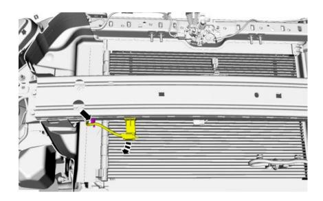
13. Position aside the ambient air temperature sensor bracket and wiring harness guide.
