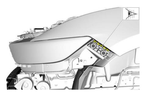
12. Inspect the fender bracket teeth for damage.
