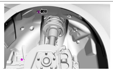
31. **NOTE:** *On both sides.* Remove the push pins.
