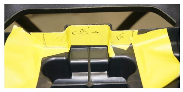
19 Just above the Reverse Lamp Opening in the Rear Bumper Cover on the Plastic Insulating Absorber Strip, Find center and mark off an area 4 ¾ inches wide or, 2 3/8 inches to the Left and Right of the Center Line.
