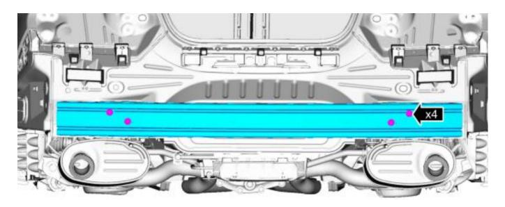
9. Remove the bolts and the rear bumper. *Torque*: **18 lb.ft (25 Nm)**
