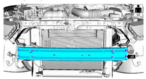
15. Remove the bolts and the front bumper. *Torque*: **18 lb.ft (25 Nm)**
