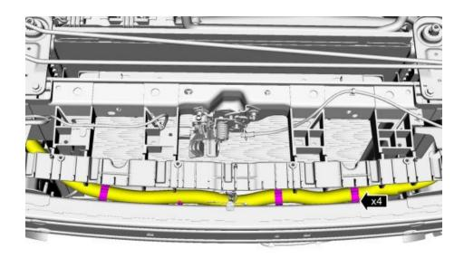
14. Separate the wiring harness guides.
