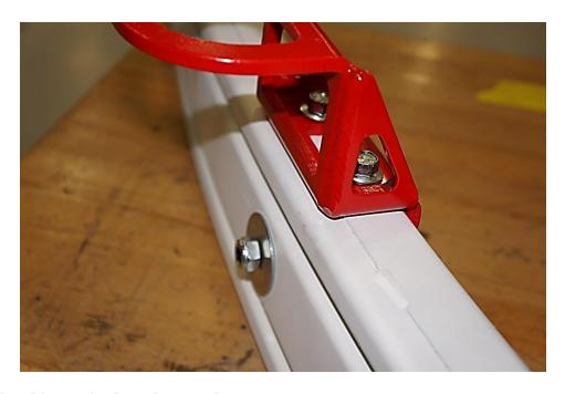
16. Bolt the Tow Ring to the Rear Bumper Beam *Torque:* **35 ft/lb (47.5 N.m)**
