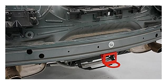
Rear Bumper Beam Re-Installed with the Ford Performance Rear Tow Ring
