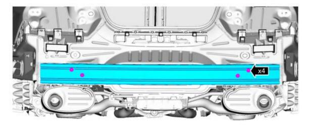
17. Install the rear bumper. *Torque*: **18 lb.ft (25 Nm)**
