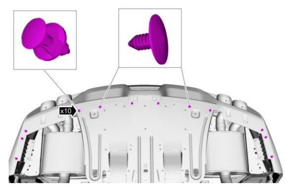
(Shelby Only) Remove the push pins and the pin-type retainers of the Rear Diffuser.
