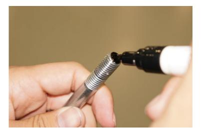
15. To Transfer the Hole to the inside of the channel on the back of the Bumper Beam, apply some paint to the end of the Bolt and, while its wet, slide the Bolt through the Hole on the Tow Ring and touch the Bumper Beam inside the channel. This is the location that you will drill a 7/16 through hole in the Bumper Beam.
