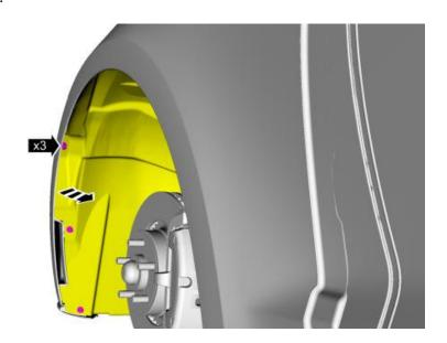
5. **NOTE:** *On both sides.* Remove the push pins and position the inner fender liner aside.
