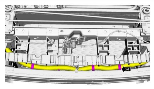
23. Re- Attach the Forward Lamp Harness to the Front Bumper Beam.
