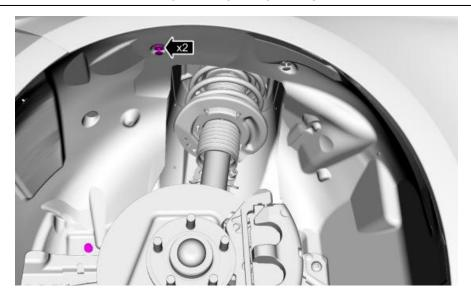
4. **NOTE:** On both sides. Remove the push pins.
