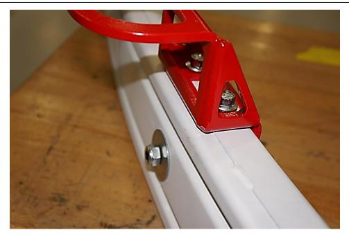
21. Bolt the Tow Ring to the Front Bumper Beam. *Torque:* **35 ft/lb** (**47.5 N.m**)
