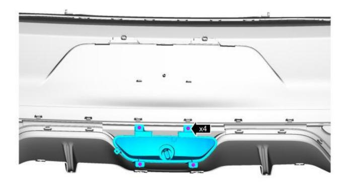
18 Remove the 4 Screws that attach the Reverse Lamp Housing to the Rear Bumper Cover then, remove the Reverse Lamp Housing. The Reverse Lamp will not be re-installed.
