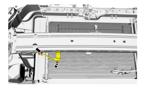
24. Install and Connect the Ambient Temperature Sensor.
