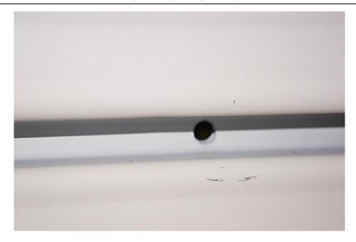
Hold Drilled through the Channel of the Rear Bumper Beam
