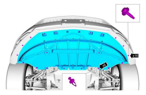
3. Remove the push pins, screws and the lower air deflector.
