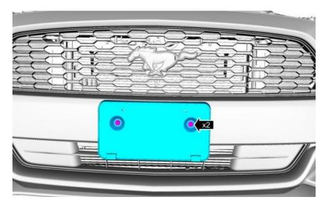
9. If equipped, remove the screws and the license plate bracket.
