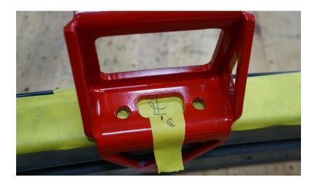
17. Find and mark the Center of the Tow Ring. Lay the Tow Ring over the Bumper Beam and align the Center Line Marks. Transfer the Bolt Holes to the Bumper Beam.
