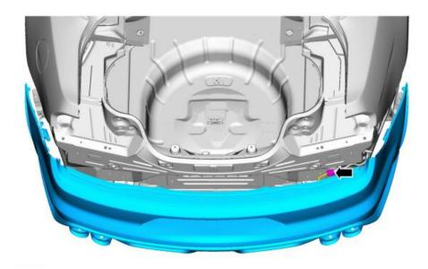
8. Disconnect the electrical connector and remove the rear bumper cover.
