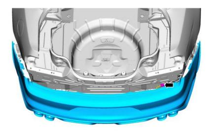
21 Re-connect the Electrical Harness and Install the Rear Bumper Cover.
