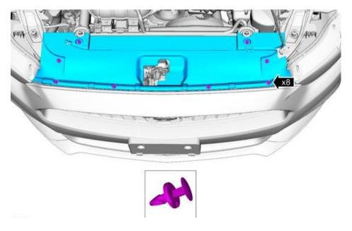
8. Remove the push pins and the radiator sight shield.
