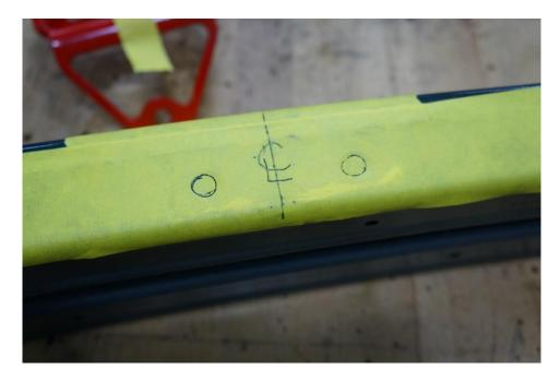
18. Your marks should look like the above Picture. Again, make sure these marks are on the BOTTOM of the Bumper Beam and drill the two (2) holes using a 7/16 bit. You will drill through two (2) layers. You will see the bit in the Center Channel on the back of the Beam when you drill through properly. (see below Picture)
