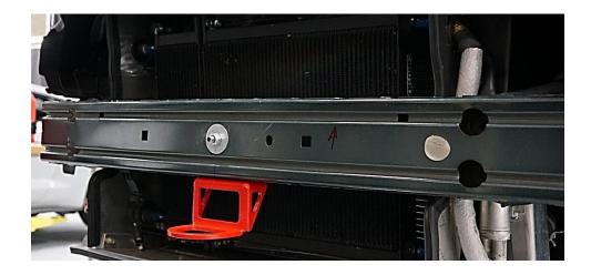
22. Install the front bumper and the Bolts. *Torque:* **18 lb.ft** (**25 Nm**)
