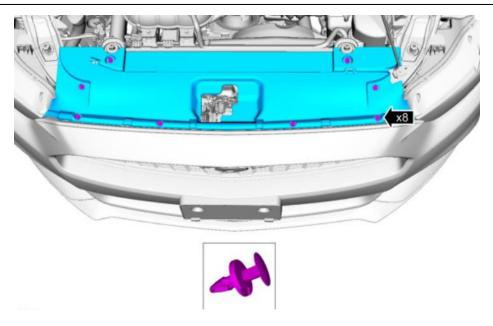
27. Install the Sight Shield and Push Pins.
