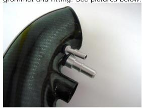
8 Attach coupler and clamps to the small end of the JLT tube and the air filter to the large end.
