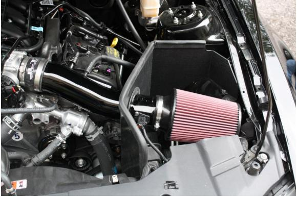
Oil Filter: The frequency you should clean your filter will depend on your driving conditions. It is recommended to check your filter at every oil change or 3,000 miles. If there is a build up of dirt as thick as the wire mesh, then it's time to clean your filter. As dirt builds up on your filter, the restriction of the airflow also increases. More frequent cleanings will improve your fuel economy and your vehicle's performance.
