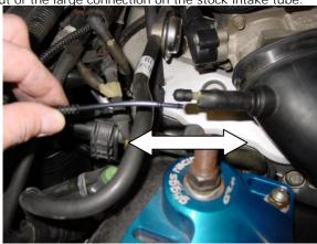
Unbolt your Mass Air Flow Sensor from the filter housing, and install the MAF filter adaptor using the supplied MAF gasket and bolts shown below. Do not reuse the screen BOLTS GO THROUGH MAF AND THREAD INTO ADAPTOR.
