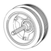
Using the Strap Wrench, install a new crankshaft pulley bolt and the washer, tighten the bolt in 4 stages:
