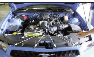
Remove the eight (8) plastic push fasteners using a small flat blade screw driver and remove the radiator support panel cover from the vehicle (to be reused).
