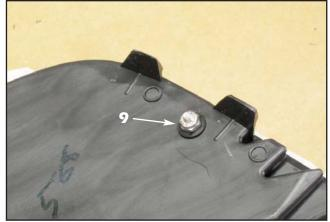
9. Carefull align the cleaned "Q" grille into the factory grille insert, making sure you do not scratch the factory grille insert. Install a black plastic washer and a 8-32 ESNA half nut onto each stud and tighten.
