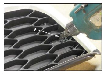
7. Use a 1/8" drill bit to drill a pilot hole where the marks were made in the factory grille. Enlarge the holes to 5/16".
