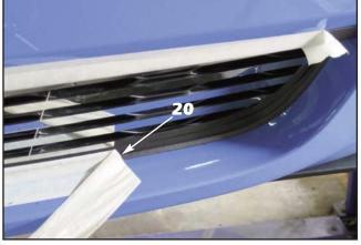
**20**. Remove the protective masking tape by pulling it back over itself to minimize tape breakage. Lift up on the "Q" grille if the tape appears to be caught underneath.
