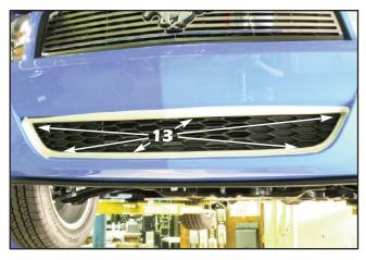
**13**. Apply protective masking tape around the lower grille opening (as shown).
