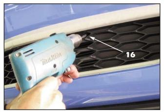
16. Test fit the lower grille. If the upper studs hit the factory grille, remove the "Q" grille and use a 5/16" drill bit to remove some of the factory plastic interfereing with the upper mounting studs. If you do not do this, the grille will not be centered in the factory opening.
