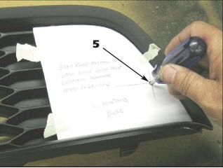
5. Carefully cut out and align the upper grille outer hole location template and tape it into place and use an awl or similar pointed tool to mark the grille at the hole locations. Keep the awl **perpendicular** to the surface of the grille for an acurate hole location.
