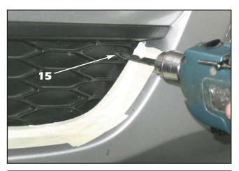
**15**. Use a 5/16" drill bit to drill through the marks made in the previous step.
