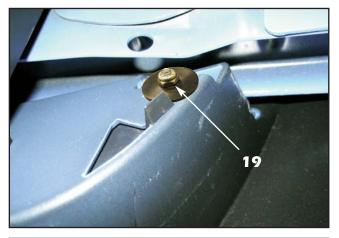
**19**. Install a large black plastic washer and a #8-32 ESNA half nut onto each outer stud and tighten.
