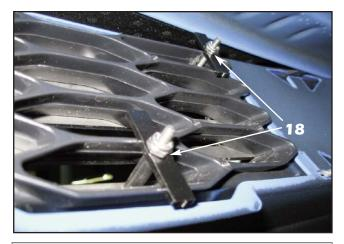
18. Align the lower grille into place, making sure that the studs protrude through the outer holes drilled in Step 15. Install the supplied rectangular mesh retainers to secure the grille to the factory lower grille.
