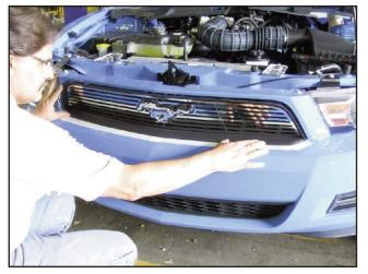
**10**. Position the grille back into the bumper cover opening and align the mounting tabs. Press firmly to engage the mounting tabs into the slots in the bumper cover.
