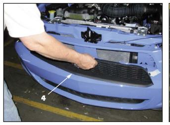
Carefully pull the factory grille insert out of the bumper cover, making sure you do not drag it across the top of the bumper cover.
