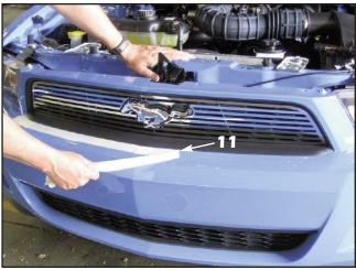
11. Carefully peel off the masking tape from the bumper cover to finish the upper grille installation.
