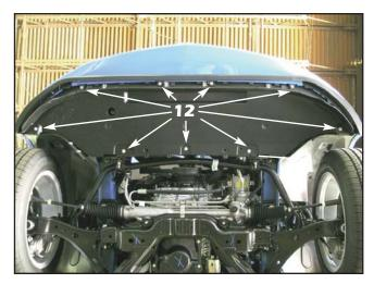
Raise the vehicle and remove the lower front aero pan 5.5mm hex screws.
