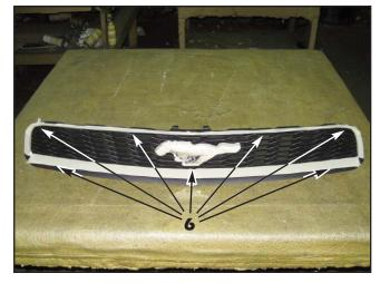
6. Carefully tape the grille insert as shown to prevent scratching the plastic during the "Q" grille installation. You must also carefully tape the raised mounting boss surrounding the pony emblem.
