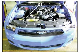
**21**. Reinstall the radiator support panel cover and the lower aero pan to finish.
