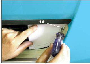
14. Using the supplied template, mark the outer stud hole locations using an awl or similar pointed tool.
