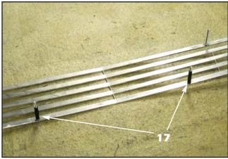
**17**. Trim the closed ends from the black cap plugs and install them onto the lower center mounting studs on the lower grille.
