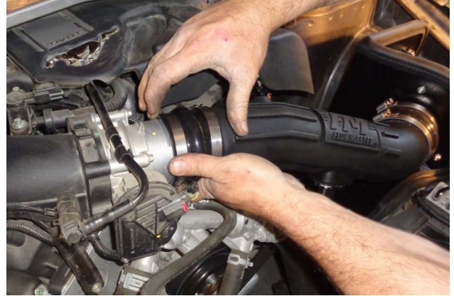
28. Install the left coupler on the throttle body.
