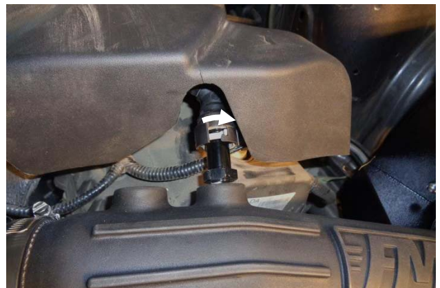
30. If your vehicle has a latching PCV fitting, secure it by pushing the latch to the right until it clicks.
