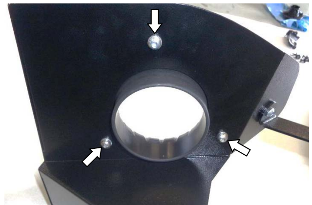
18. Assemble air filter adapter (3) to heat shield using M6 screws (22), lock washers (11) and flat washers (23).
