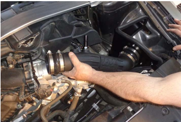
26. It is recommended that the assembled intake tube be installed as follows. First, install the right coupler on the filter adapter.
