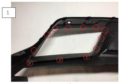
Locate the mounting tabs on the diffuser.
