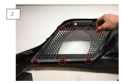
Align the mounting tabs with the insert. Press on the insert onto the diffuser. Ensure all the tabs clip into place.
