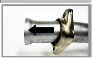
Slide the flared flanges over the head pipes so that the flared end of the flanges match the flared end of the head pipes as shown.
