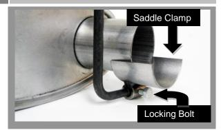
Use the hanger and saddle clamp for the outlet of the muffler. Slide the hanger through the corresponding rubber grommet on the chassis then snug the hanger into the saddle clamp and tighten the locking bolt to hold the hanger in place.
