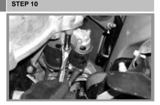
Unbolt and remove the starter from the bell housing.
