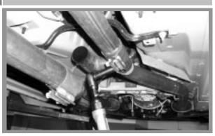
Separate the cat-back system by loosening the 2 nuts on each band clamp and prying the locking tabs up with a small screwdriver while sliding the clamp towards the rear of the car.
