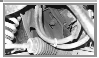
To avoid damage to the header coating or paint in the engine compartment it may be necessary to raise the right side of the engine while installing the passenger side BBK Header. The motor mount is connected to the vehicle with 1 nut, easily accessible from under the front of the vehicle.
