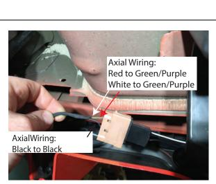
**Step 3**Connect the Raxiom wiring to factory wiring harness as follows:
