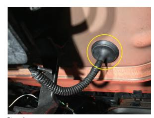
**Step 4**Locate the body grommet on the bottom of the trunk. Carefully pierce only the body grommet so that you can feed the yellow and red wires from the reverse light into the trunk.
