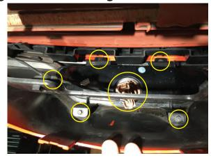
**Step 2**Pull the valance down to gain access to the (4) factory reverse light screws (7mm). Un-clip the plug on the factory light and remove the harness from the housing. Install the Axial light the same way the stock light came out.
