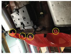
**Step 1**Begin by removing the (2) screws and (2) clips securing the lower bumper valence.
