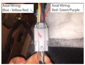
**Step 8**Using the t-tap wire splices, tap the following wires:
