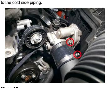
**Step 10:**Once the pipe is installed rotate the pipe/couplers to achieve the best fit. Ensure the piping isn't making contact
