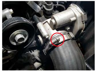
**Step 8:**Loosen the factory hose clamp that secures the cold side piping to the intercooler.
