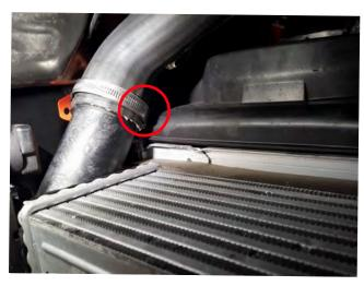
**Step 9:**Loosely install the supplied silicone couplers and clamps
