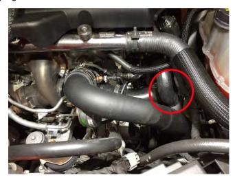
**Step 7:**Loosen the factory hose clamp that secures the cold side piping to the throttle body.
