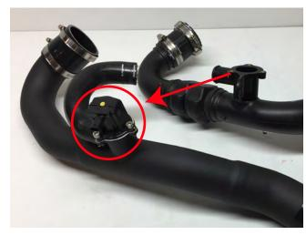
**Step 6:** Install the SR intercooler pipe. Re-attach the bypass valve plug and hoses.
